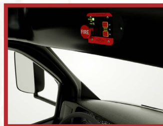
SMVS Control Panel
